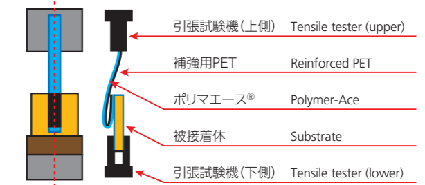
引張試験時概略図 Schematic diagram of tensile test
