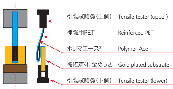
引張試験時概略図 Schematic diagram of tensile test
