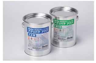
A 5kg set of the resin (A-component) and a hardener (B-component). It can be used to fill in cracks and gaps and will not be washed away by water due to its clay-like consistency. At an outside temperature of 23°C, it hardens in about 45 minutes with a solidity of 80°C.
