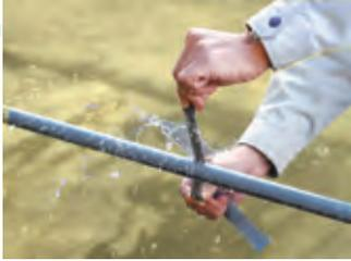
**Rubber tape** to prevent leakage from pipes, etc.
