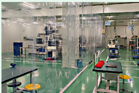
Partitions installed between the molding work area (left) and the back-end process area (right) to control air conditioning
