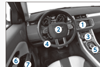
Automotive input devices ① Audio/navigation display ② Steering switch ③ Center console switch ④ Engine start/stop switch ⑤ Electronic shifter switch Electric parking brake switch Haptic switch ⑥ Seat memory switch ⑦ Power window switch
